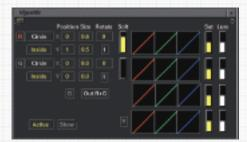
Once "V1" is pressed and the window open, the R and G channels are used to select areas of the picture. There is no colour selection, only the shapes are used; R, G, B and Y are channel names only. The lower orange display (SCC) will show the shape controls, in the same order as for Mega 1. As the R and G channels have there own shape generators, the knobs control whichever of these two channels is currently selected.
