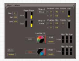
The Mega 1 secondary channel can be chosen from the white keys at the bottom of the panel, marked R,G,B,Y,C and M; the current channel selector key will be illuminated green. Although these channels are set so the colours (vectors) they initially effect roughly correspond to the label on the white key, any channel can be made to work on any colour; the labels (RGBYCM) should be regarded as names.
