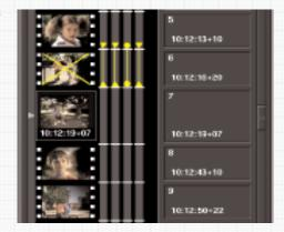
The current code is shown between the two most central thumbnails Fig. 68 (this cannot be permanently changed, to put the code nearer the top or bottom). In telecine mode only, the type of code displayed can be changed in the User setup window, or temporarily changed by holding down the telecine transport key for a couple of seconds, to toggle through the different options. These are: Filmcode (time and frames); Feet and Frames; Frames only and Timecode.
